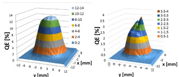
Figure 1: QE maps of Cathode #198 (Cs<sub>2</sub>Te) as newly produced (left) and used in the RF photoinjector (right).
