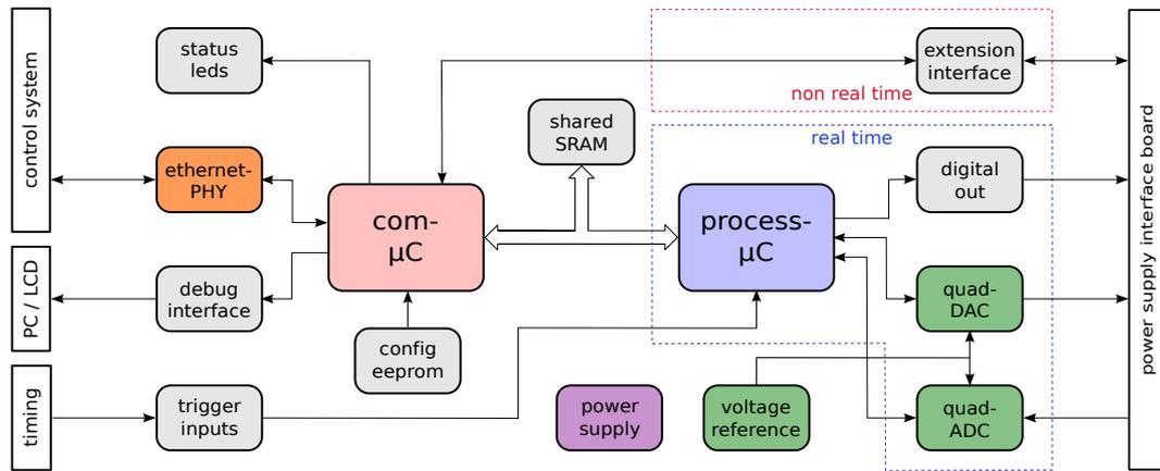
Figure 2: Block diagram of the hardware modules.
