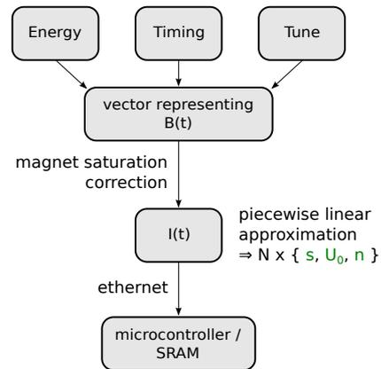
Figure 4: Calculation of ramp data.
