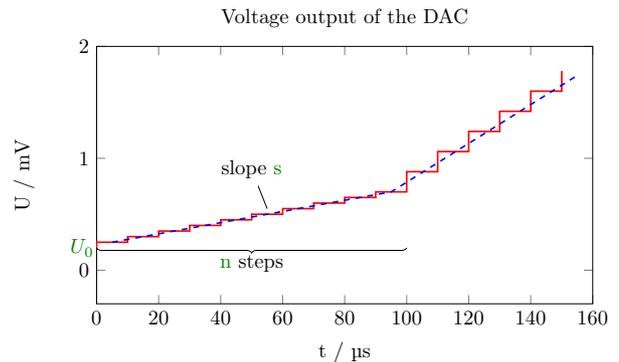
Figure 5: Piecewise linear approximation (shown in dashed blue) of the desired non-linear function for  $I(t)$ , represented by  $U(t)$  (shown in red).
