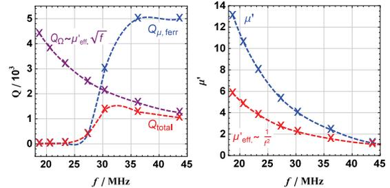
Figure 5: Left:  $Q_{\text{total}}$ ,  $Q_{\mu, \text{ferr}}$  and  $Q_{\Omega}$  vs. frequency. Right:  $\mu'$  and  $\mu'_{\text{eff}}$  vs. frequency.
