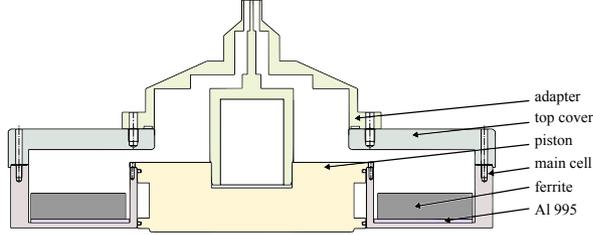
Figure 3: 1-port reflection measurement setup.
