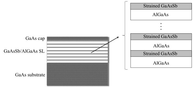
Figure 5: Schematic structure of GaAsSb/AlGaAs SL material.
