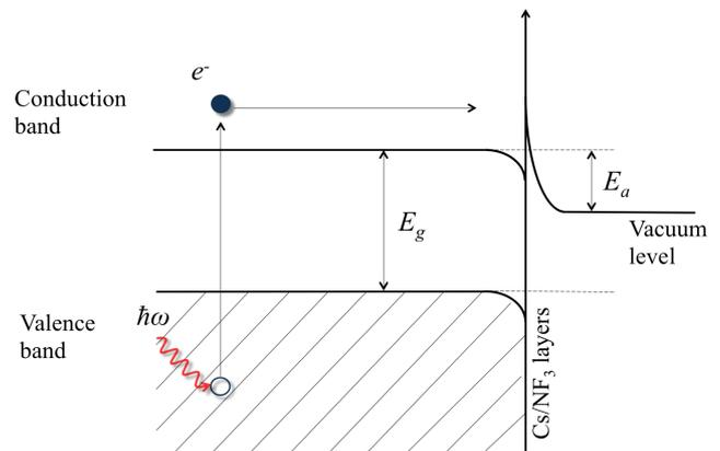
Figure 1: Photoemission from GaAs activated to NEA by putting layers of  $Cs$  and  $NF_3$  on the surface of photocathode: photoexcitation of valence electrons into the conduction band; transport of electrons to the surface; emission of electrons into the vacuum.
