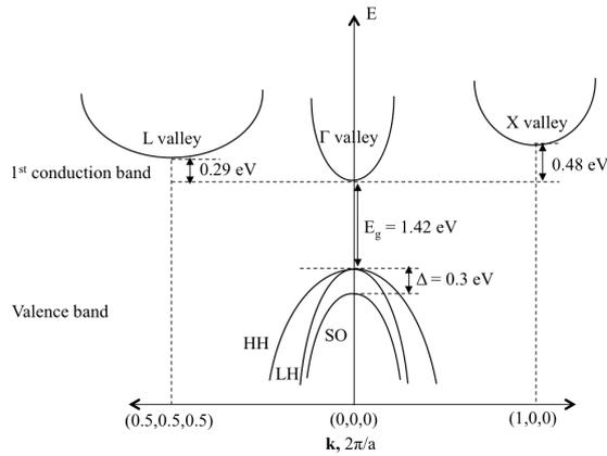
Figure 2: Band structure of GaAs ( $T = 300$  K).
