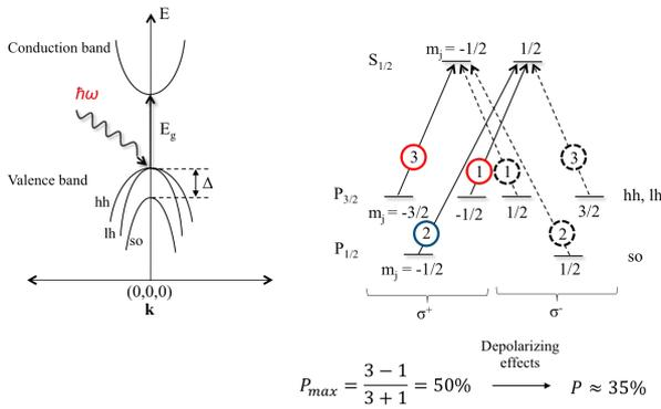
Figure 3: Electromagnetic transition probabilities at the  $\Gamma$  point of unstrained GaAs: positive  $\sigma^+$  and negative  $\sigma^-$  helicities correspond to transitions during excitation by right-polarized (solid lines) and left-polarized (dashed lines) photons, respectively; numbers inside the circles indicate the relative strength of transitions; different colors indicate transitions under excitation by photons of different energy.
