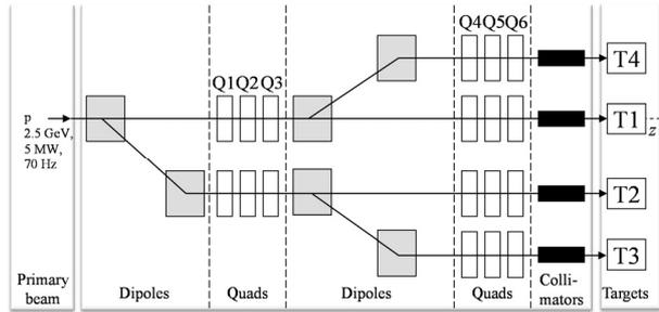
Figure 4: Principle of config2.
