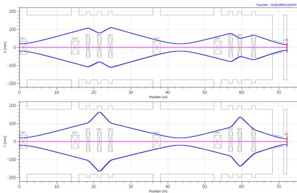
Figure 5: Beam envelopes ( $4\sigma$ ) – T3 axis (config2).
