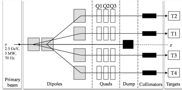
Figure 1: Principle of config1.
