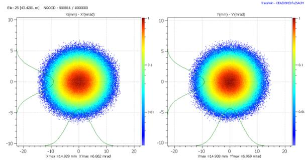
Figure 3: Beam output phase-space distributions in  $(x, x')$  and  $(y, y')$ ; T1-T3 beam lines of config1.
