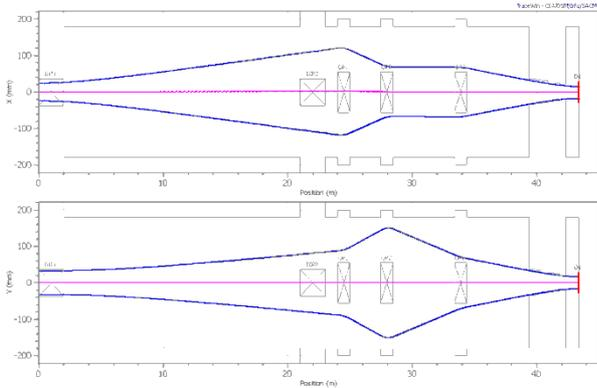
Figure 2: Beam envelopes ( $4\sigma$ ) – T1 axis (config1).
