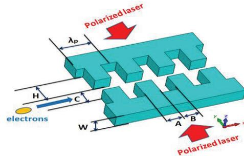
Figure 1. Schematics of a dielectric grating structure.
