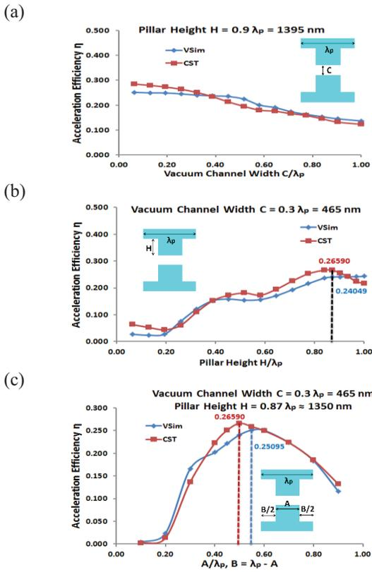
Figure 3. Acceleration efficiency  $\eta = G/E_p$ , where  $G$  is the average acceleration gradient and  $E_p$  the peak electric field in the grating structure as a function of vacuum channel width  $C$  (a), pillar height  $H$  (b) and pillar ratio  $A/\lambda_p$  (c).
