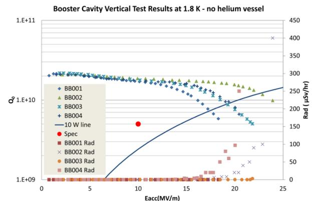
Figure 3: The  $Q_0$  vs Eacc curves for the four booster cavities for the bERLinPro project as measured at 1.8K in the JLab VTA. The design specification for the accelerating cavities is shown by the orange circle and the 10 W dissipated power line is shown by the solid blue line.
