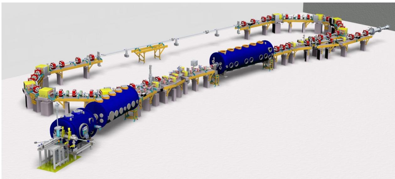
Figure 1: The bERLinPro Energy Recovery Linac machine layout.
