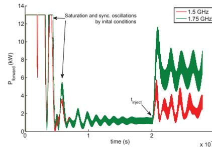
Figure 5: Required RF power due to initial synchrotron oscillations, following steady state and deviation by 1.2 mA beam injection in three long buckets.
