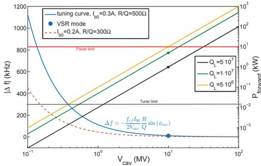
Figure 1: Optimum tuning curve for reactive beam-loading for the VSR (blue curve) and a lower  $R/Q$ -reduced intensity scenario (brown curve) as well as the required power with optimum detuning for different  $Q_L$ . Limits of the tuner and power source are given by the horizontal lines.
